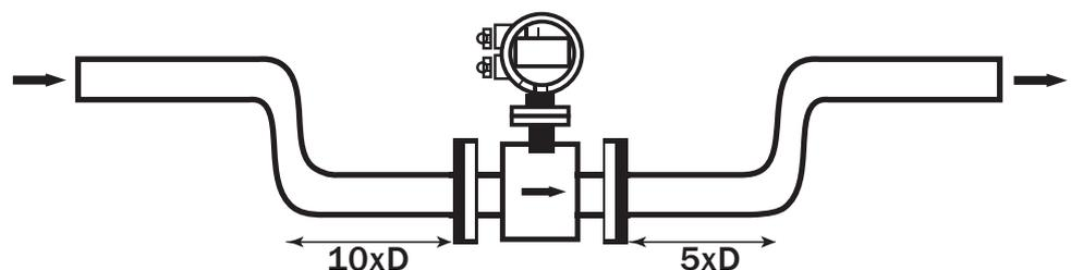
D= Diameter of Flow Meter in Inch
